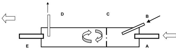
**Figure 2** Custom made mixing chamber. (A) Gases from 'CPAP driver' upstream. Pressurized and humidified oxygen mixture 'driving gas'. (B) Injection port for NO in nitrogen injected into main gas stream. (C) Baffle, producing turbulence to insure rapid mixing (D) 24-gauge midstream gas sampling port. (E) Exit port for mixed gases to 'CPAP generator' downstream.
